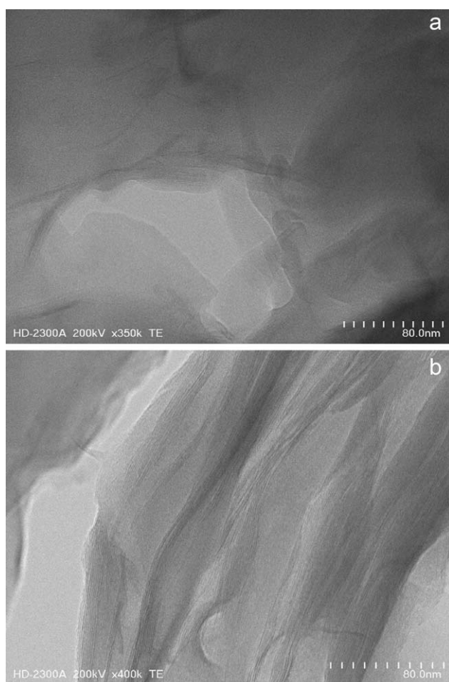
Figure 3 TEM images of PET/MMT nanocomposites prepared through (a) 0.5 wt % clay ES addition and (b) 0.6 wt % clay PC addition.
